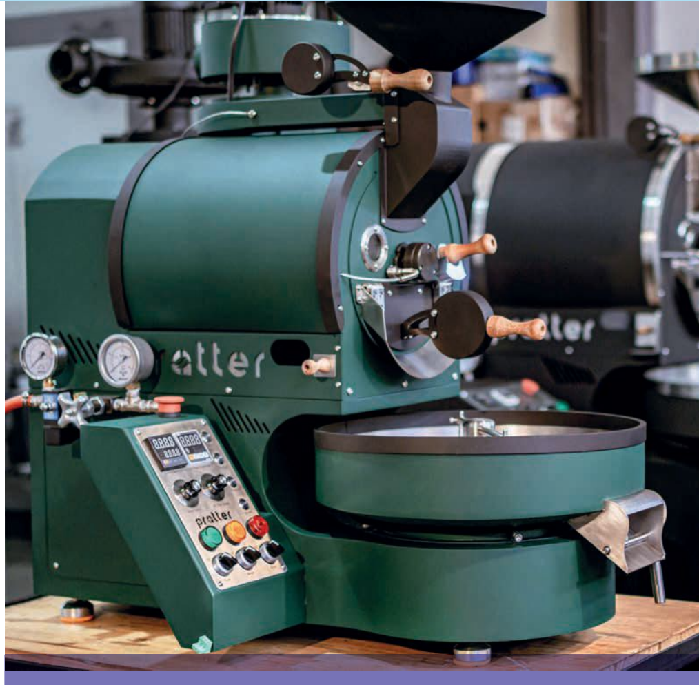
Right: An Indonesian coffee roaster opted for Optidrive E3 VFDs to control its gear motors
